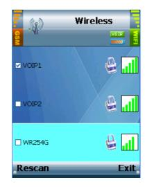
4 Select **Exit** when WLAN connection successfully, or press left soft key to **Rescan** for connecting again.
