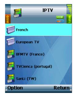
2 To turn on the channel, you can press **Select** in **Option**, or press **Center key** to activate. You might be requested to enter a password if necessary.
